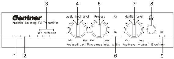
Figure 6. TX-37A front panel controls
