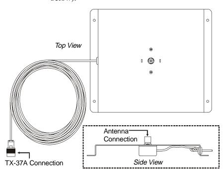
Figure 3. Remote antenna connection
