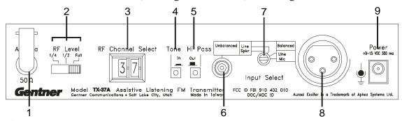
Figure 2. TX-37A back panel controls
