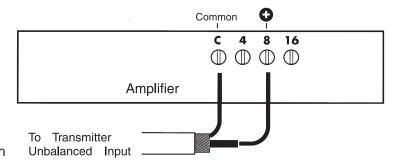
Figure 4. Amplifier connection
